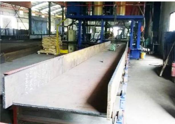
**2** MÁY HÀN DẦM TỰ ĐỘNG, LOẠI NẰM
